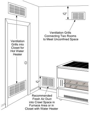
Figure 15 - Ventilation Air from Inside Building
